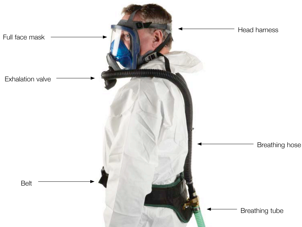
Figure 15 Fresh air hose (FAH) breathing apparatus
