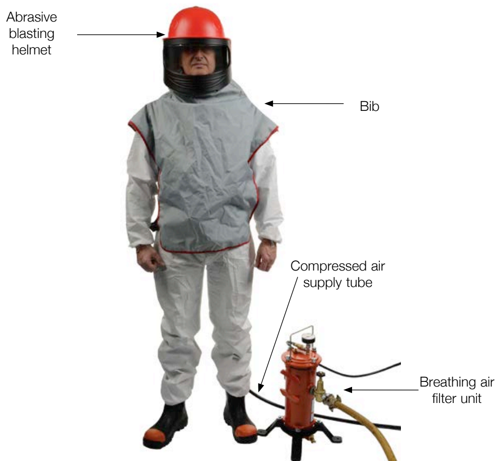
Figure 19 Constant flow airline breathing apparatus with hoods/helmets
