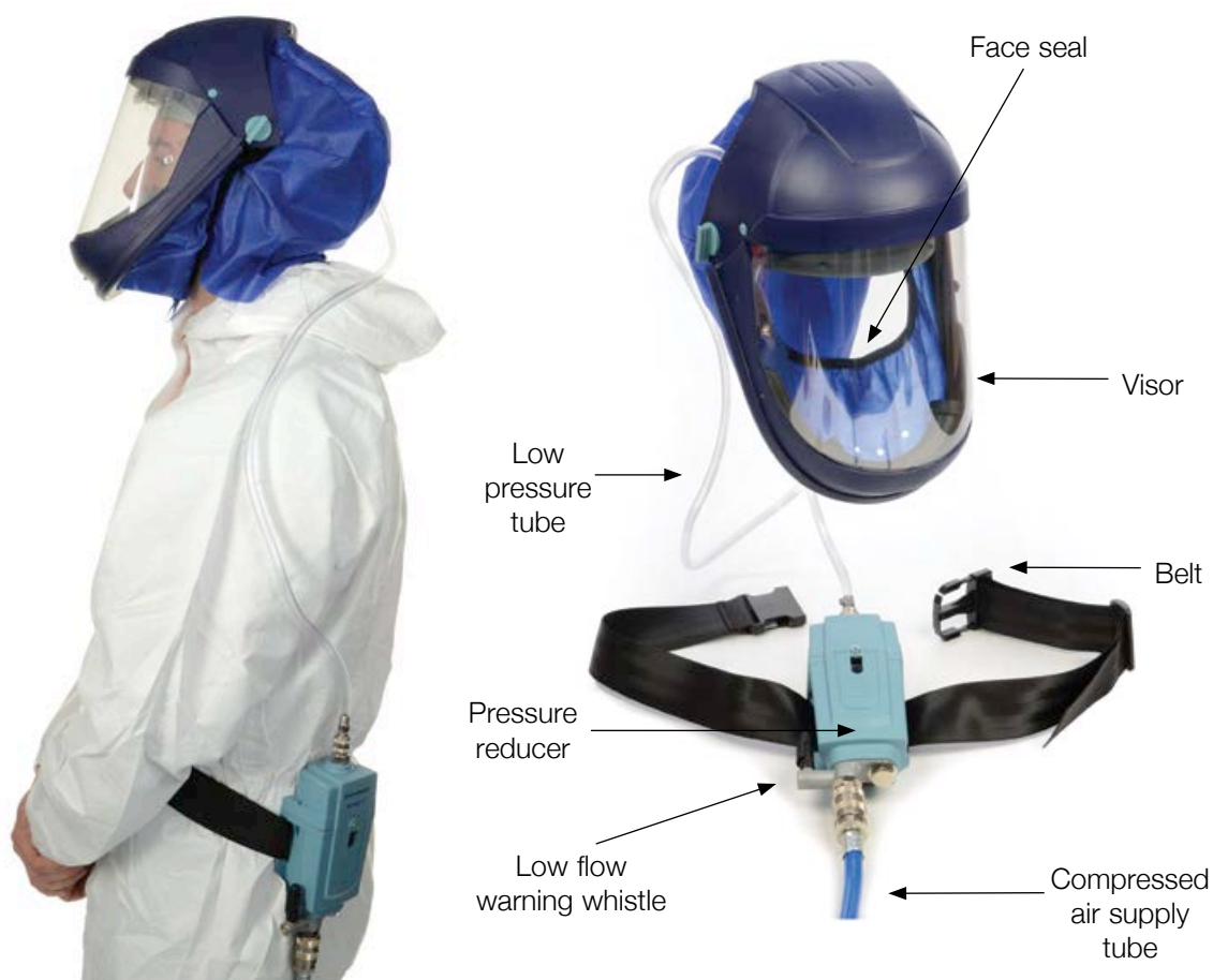
Figure 18 Constant flow airline breathing apparatus with hoods/helmets – light duty
