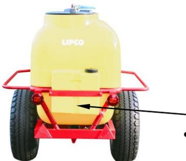
The hand washing tank must be filled with fresh water only and is used for washing the operator's hands after spraying. (Fig. 8)
