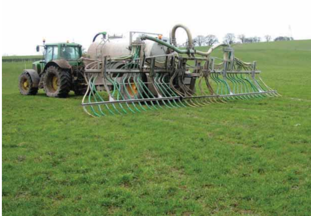
Injection of slurry to reduce ammonia emissions
