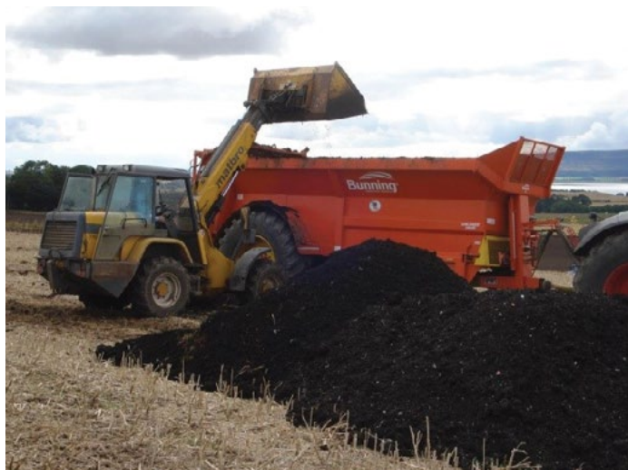
Figure 4. Compost being loaded into a modern rear-discharge spreader
